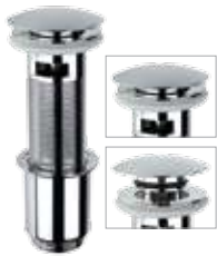
905CCXL114 Scarico automatico con sistema click-clack, 1" 1/4, tappo grande, con troppo pieno, versione extralunga. Automatic pop-up waste, click-clack system, 1" 1/4, big plug, with overflow, extralong version.
