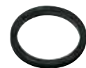
Guarnizione in gomma anticalore (EPDM) 755H, Ø 44,5x36x4, per resistenza filettata. Oring washer in EPDM, heating resistant, 755 H mm. 44,5x36x4, for threaded heating elements.
