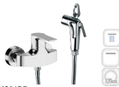
EYC31DP Miscelatore monocomando esterno doccia, interasse 100 mm, con doccetta shut-off e flessibile cm 120. Wall mounted single lever shower mixer, interaxis 100 mm, including shut-off and flexible hose cm 120.
