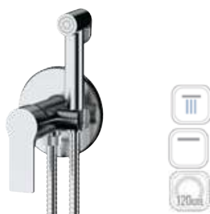
EY65W Miscelatore incasso per shut-off con supporto doccia/presa acqua integrato, attacco conico da 1/2", con doccetta shut-off e flessibile cm 120. Built-in shower mixer with integrated shower holder/water punch on flange, with 1/2 connection, with shut-off and flexible hose cm 120.
