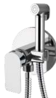
I65W Miscelatore incasso per shut-off con supporto doccia/presa acqua integrato, attacco conico da 1/2", tutto in ottone, con doccetta shut-off e flessibile cm 120. Built-in shower mixer with integrated shower holder/water punch on flange all in brass, with 1/2 connection, including shut-off and flexible hose cm 120.
